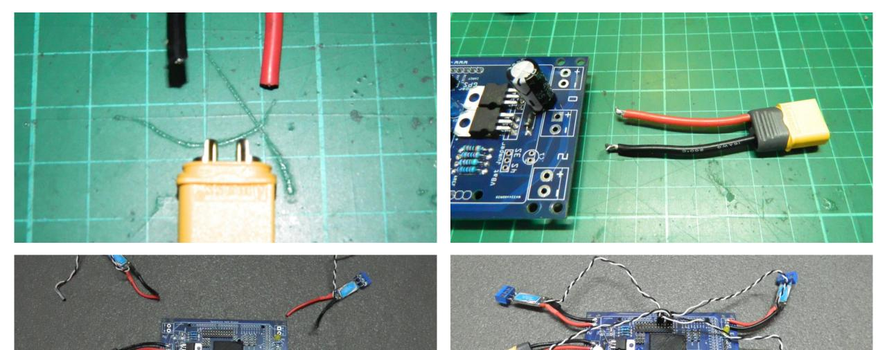
Ensure all expose contact can be isolated or insulated to prevent shorting especially ESC terminals
