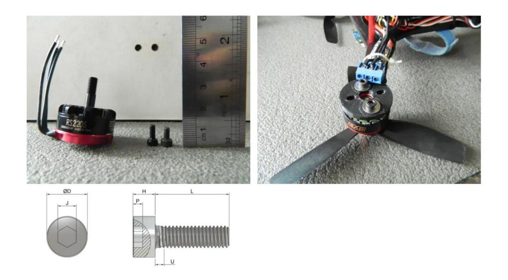
Note: this frame is design to use M3 bolts with thread length of 6mm with washer as fittings included in the set (use the shortest bolt that came with the motor set)
