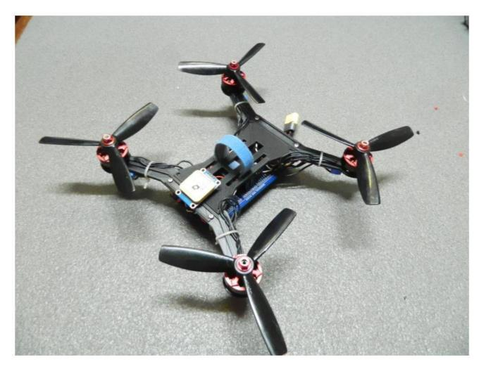
Once all the hardware been calibrated tune and setup you may zip tie the ESC and Tape insulate all the Solder Pads to prevent Shorting
