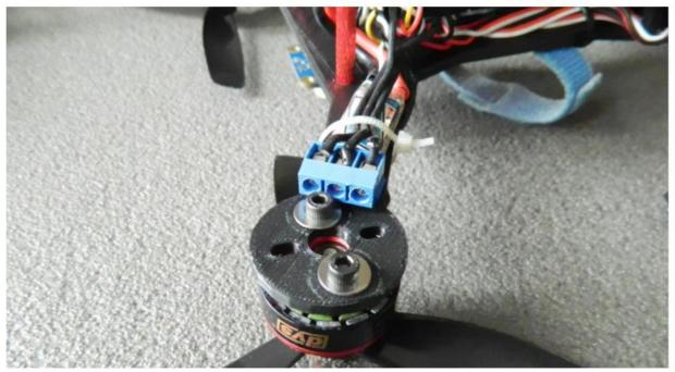
Use the 6mm M3 Bolt provided (short one) and install with washers
