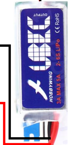
BEC or Buck converter supplying extra power
