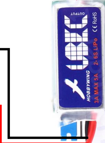
BEC or Buck converter supplying extra power
