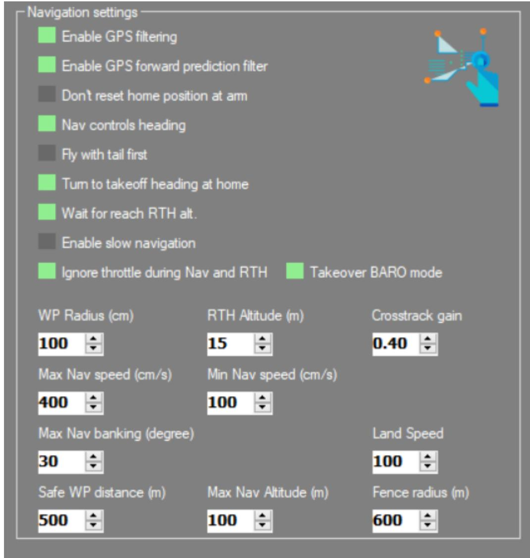
**WP Radius** – the radius of the area the Pos PID with trigger it has reach the waypoint
