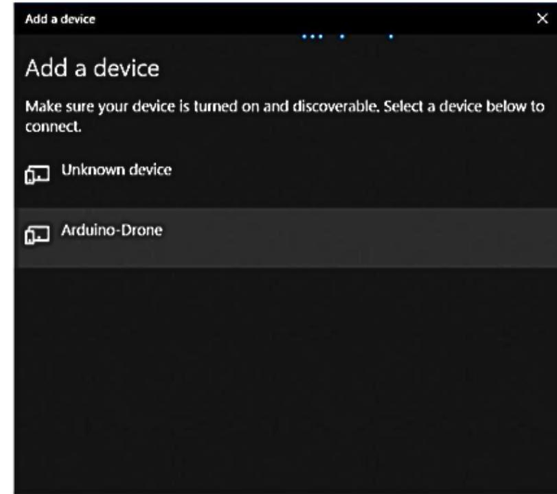
Adding Bluetooth on Windows Device Manager look for Arduino-Drone BT device
