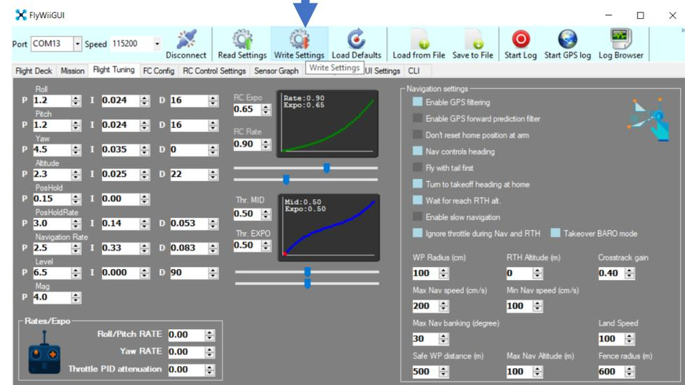
Load the PID file and Write settings after changes made in any of the parameters
