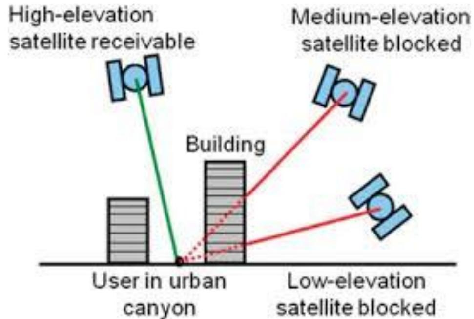
**Note : GPS require a clear open area to get a proper fix and accuracy minimum 7 satellites but 10+ are Ideal**
