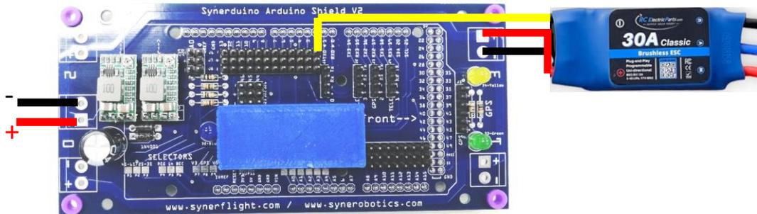
Reg in – to use the onboard power supply to run the board up to 3A
