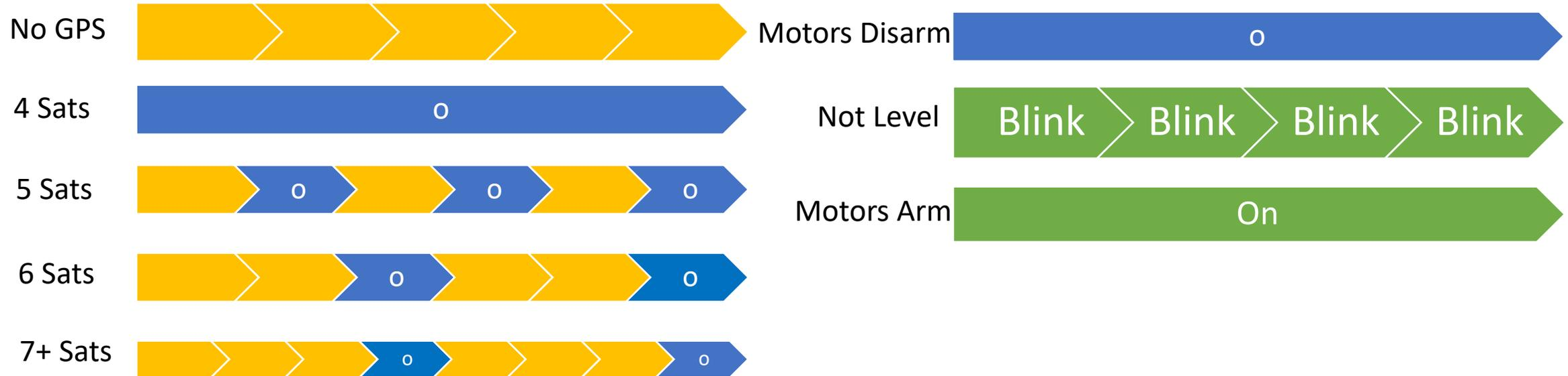
indicate a valid GPS fix by flashing the LED
