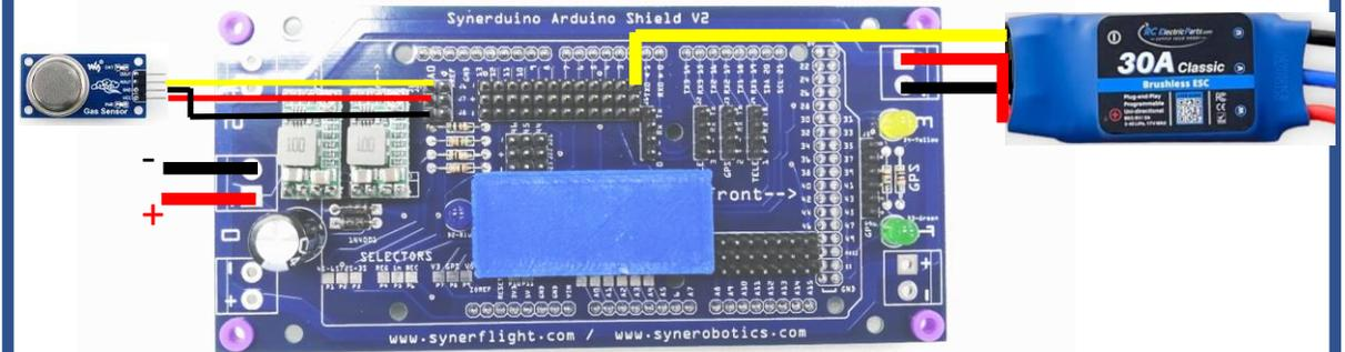
BEC in – if your using External BEC or ESC Bec to provide much needed Power to run Servos and External sensors and Companion Hardware **NOTE: Synerduino only support 5V input from BEC**
