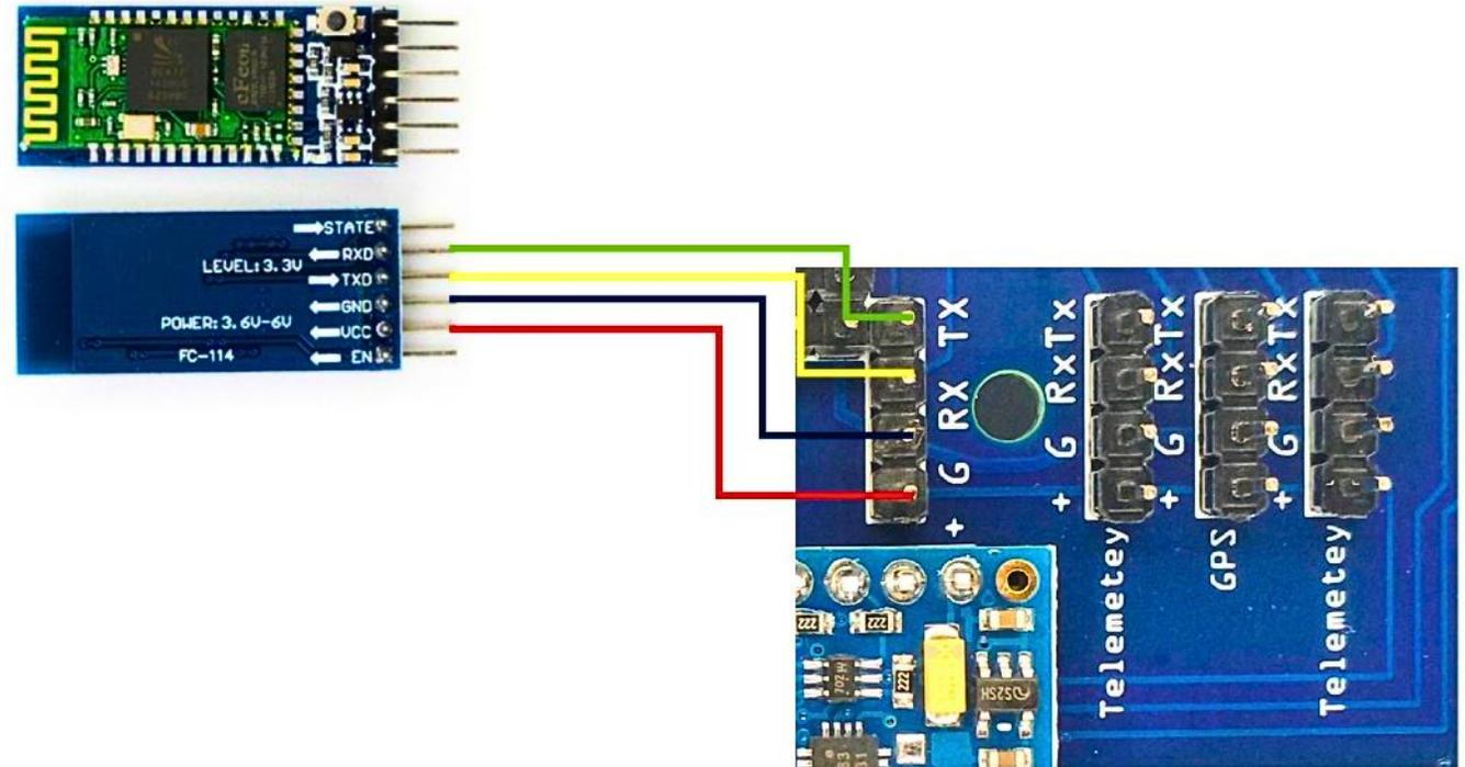
NOTE: DOUBLE-CHECK THAT THE WIRE COLORS MATCH THESE MARKINGS. INCORRECT INSTALLATION OR POLARITY MAY DAMAGE THE ARDUINO BOARD. THE BLUETOOTH MODULE IS PRESET TO A BAUD RATE OF 115200 FOR YOUR CONVENIENCE, BUT YOU MAY CHANGE THE SETTINGS IF NEEDED.
