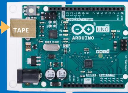
Add tape to the top-left side of the Arduino 2560 MEGA/UNO 328 board to cover the metal part.
