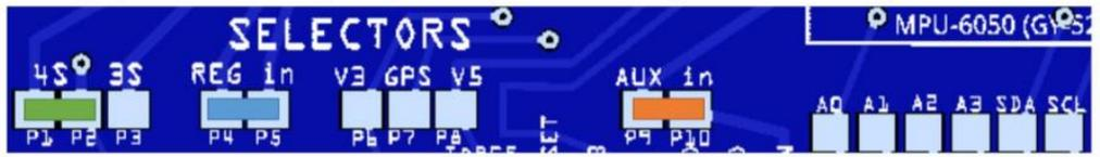
For those who would use the build in battery monitoring circuit upto 4s lipo ensure the Cell Count and Aux in is jumped before powering up
