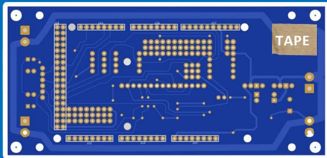
Add tape to the top right side corner at the back of the Synerduino board.
