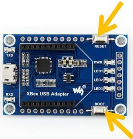
GET THE USB MODULE WITH BOOT AND RESET BUTTON AS YOU MAY NEED TO RESET THE XBEE WHEN UPDATING FIRMWARE
