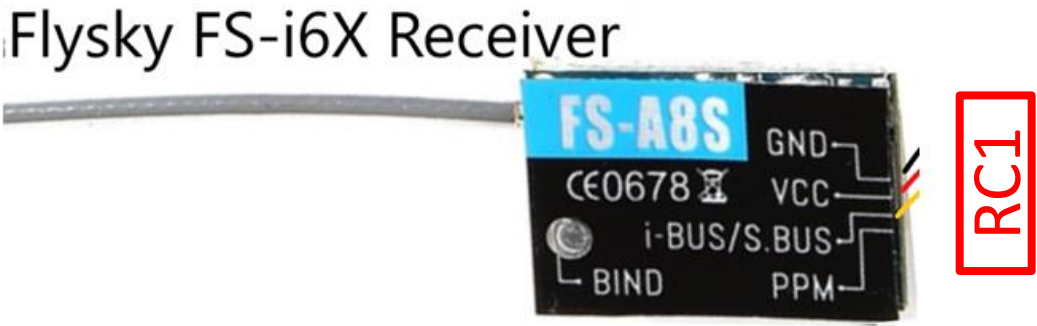
Receiver : Connect to RC1 / UART2
