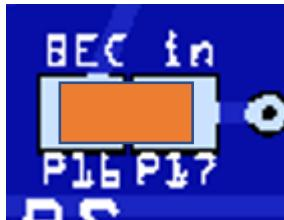
P16-P17 : BEC –this is use if you have a BEC powering through the ESC w/UBEC or an Standalone UBEC or Buck Converter Plug into S2 Pin **BEC input is 5V**
